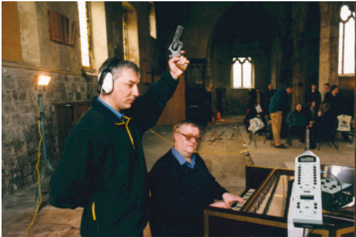
Acoustic tests in March 1998 confirmed that the best use of the excellent acoustics would be to keep the church as one performance space, as the plan below
